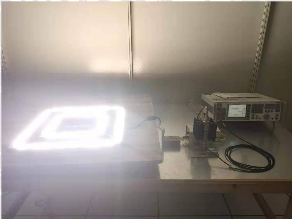
7.9 Photograph – Injected Currents Immunity Test Setup
