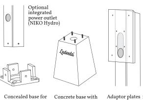
Concealed base for invisible mounting on concrete base or paved surface
