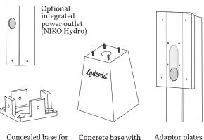
invisible mounting on concrete base or paved surface
