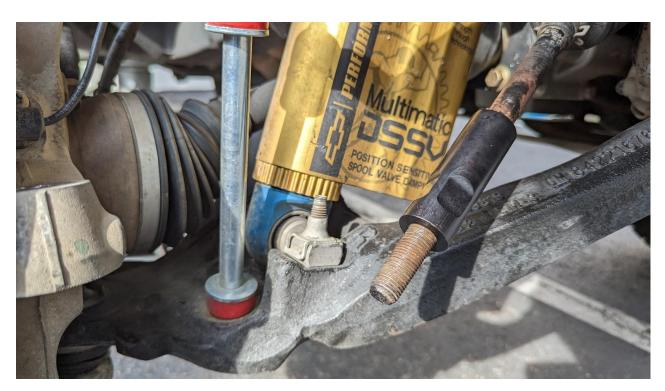
9) Counting the number of turns as you go, thread the tie rod end assembly onto the tie rod and insert into the knuckle using provided washer and nut
