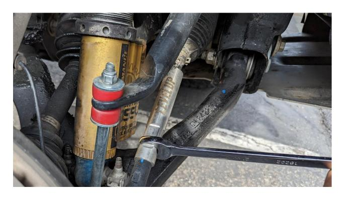
4) Using 10mm wrench to hold hex and 21mm wrench, loosen tie rod but do not remove nut all the way
