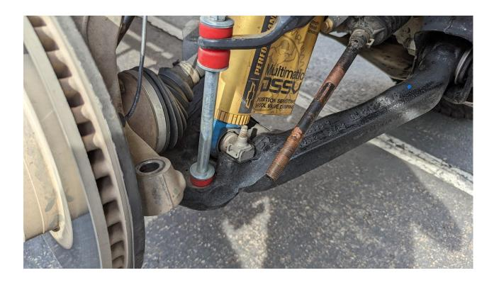
8) Install the sleeve on to the tie rod
