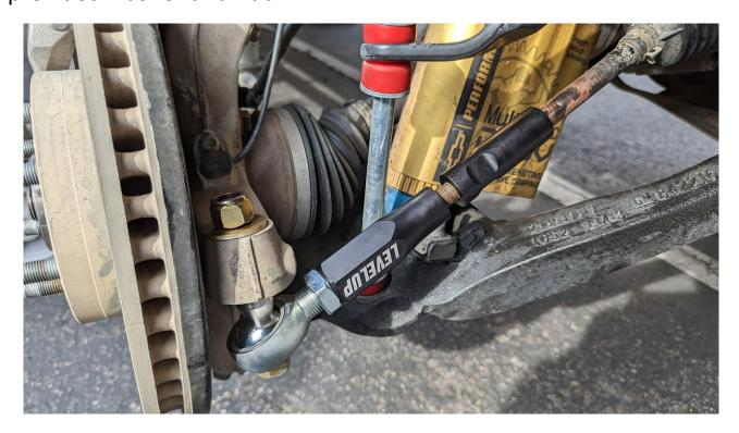
10) Torque the nut to 26 lb\*ft and then tighten the nut an additional 85-95 degrees
