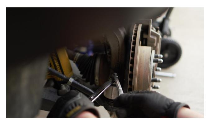
5) Using ballpeen and weighted hammer lightly tap tie rod are to break taper loose if necessary
