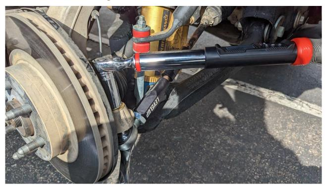
11) To align loosen tie rod sleeve with flats (A below) using 21mm wrench and adjust the tie rod using the flats (B below), do not align using the nut on the rod end
