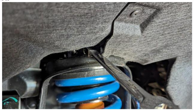
11) Using an 18mm wrench loosen the upper control arm ball joint nut and remove the ball joint from the knuckle
