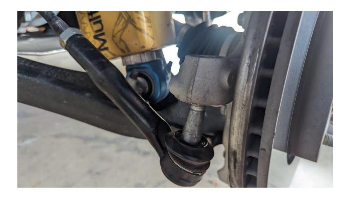
7) Remove wheel speed sensor wire from upper control arm
