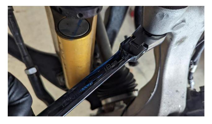
12) The shock assembly can now be removed from the vehicle
