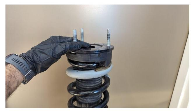
15) Remove the boot, being sure to leave the bump stop and properly put the upper mount adapter into place, making sure it sits flat
