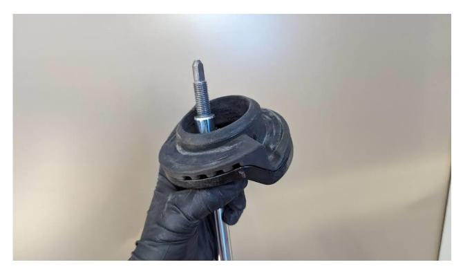
17) Next install the threaded sleeve, springs seat, washer and reinstall the bump stop cap as shown below
