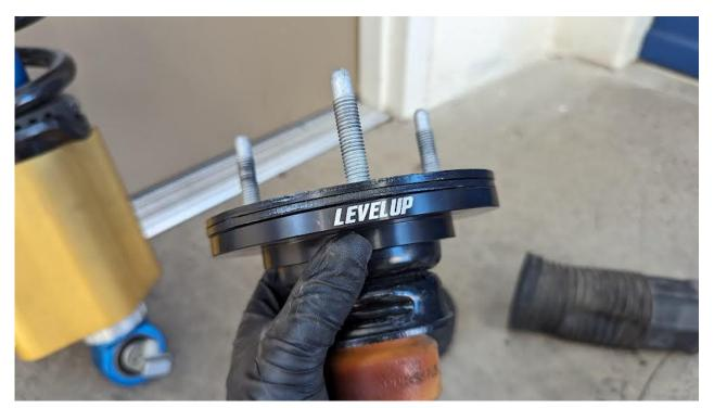
16) Remove the spring, bump stop cap and the lower spring seat
