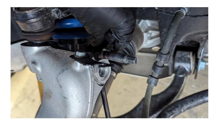
10) Using a 15mm ratcheting wrench remove the 3 upper shock nuts
