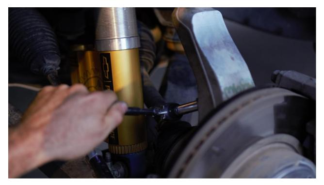
31) Reinstall and tighten tie rod ball joint using 10mm and 21mm wrenches
