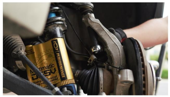
11) Using a jack (or buddy) support the lower control arm and loosen the last few turns on the upper ball joint nut being careful not to let the knuckle hang on the brake line
