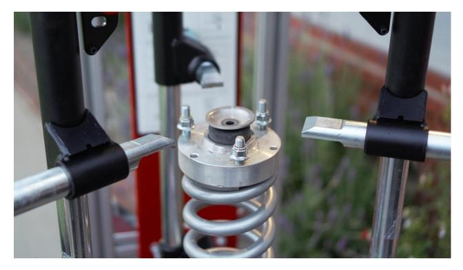
24) Compress spring and slide shock with washer, bushing, and sleeve installed into spring and top mount. Be sure single bolt on top mount is oriented in same direction as DSSV Reservoir as shown. The closer these are lined up the easier reinstall will be
