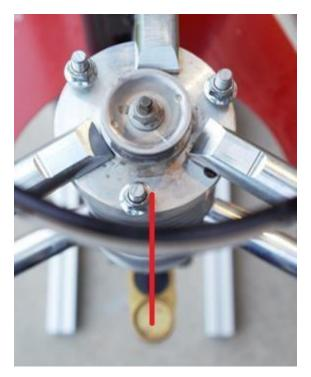
25) Tighten nut using 15mm and 6mm wrenches
