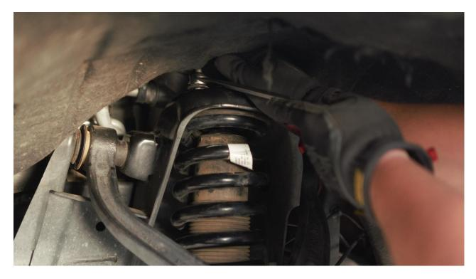
9) Use a 15mm deep socket to loosen the two bottom shock bolts
