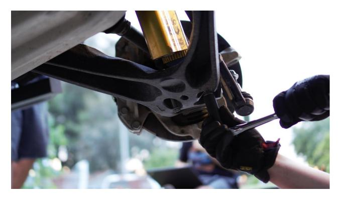
29) Install provided nuts onto upper shock mounts and tighten using 15mm ratcheting box wrench
