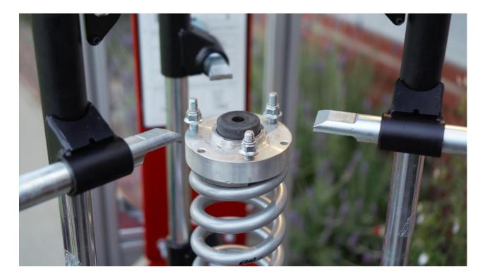
23) Place OEM washer onto bushing as shown
