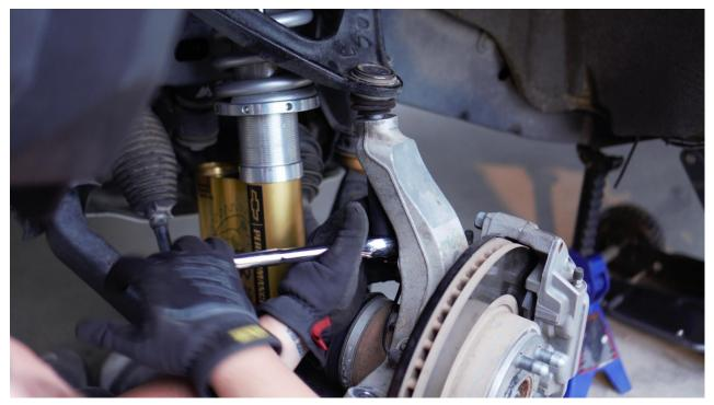
28) Reinstall and tighten lower shock bolts using 15mm socket
