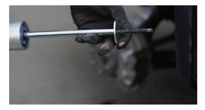
19) Place provided bushing on top of washer, on shock shaft
