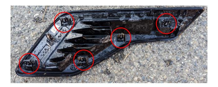
5) Place the metal clips into the fender, in the holes shown below
