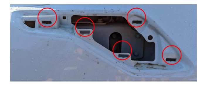
6) Carefully push the new carbon fender vents into the fender making sure the tabs are properly aligned
