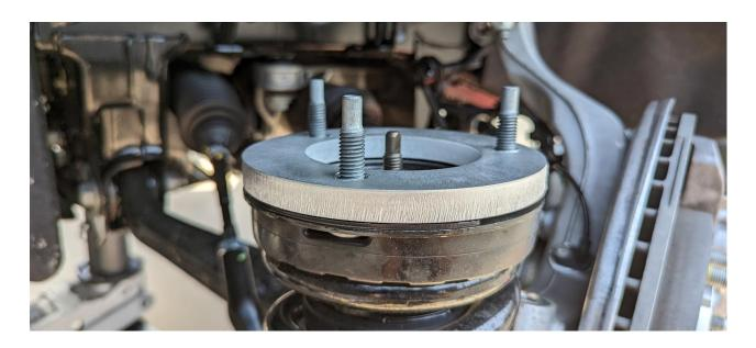
15) Reinstall the shock into the vehicle
