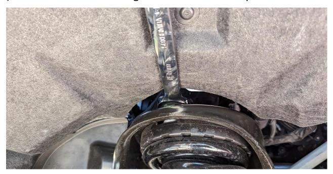
8) Using an 18mm socket loosen the upper control arm ball joint, separate the ball joint using the two hammer method or a ball joint separator and undo the upper control arm from the knuckle
