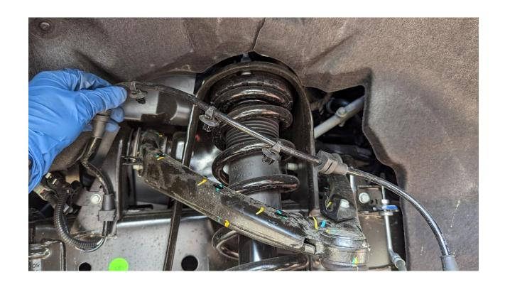
6) Using a 21mm & 10mm wrench loosen the sway bar end nut and remove it from the knuckle
