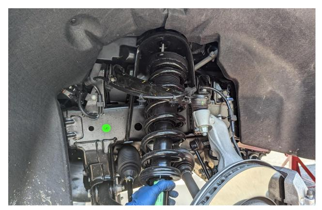
10) Using a spring compressor, compress the spring and remove the upper mount, pay close attention to the upper mount orientation, it is best to mark it relative to the shock to make reassembly easier
