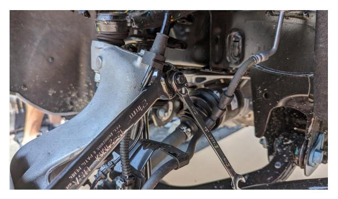
7) With an 18mm ratcheting wrench loosen the top shock nuts
