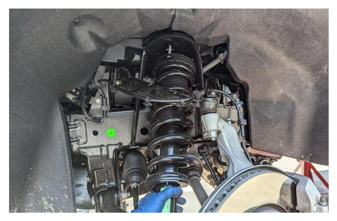
10) Reassemble the shock making sure upper mount is properly aligned in relation to the lower shock mount
