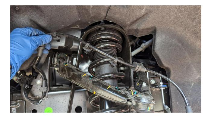
6) Using a 21mm & 10mm wrench loosen the sway bar end nut and remove it from the knuckle
