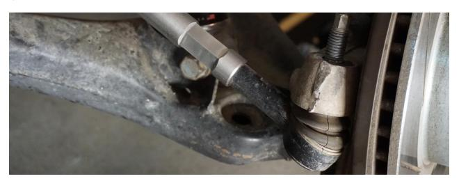
14) Replace tie rod end nut and tighten
