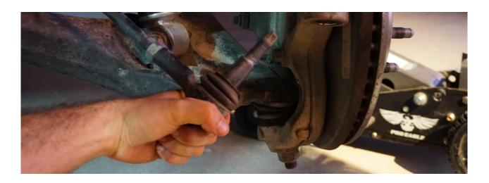
7) Unthread the tie rod end from the tie rod, being sure to count the number of turns it takes to remove the tie rod end
