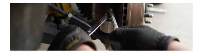
5) Using ballpeen and weighted hammer lightly tap knuckle near tie rod to break taper loose if necessary
