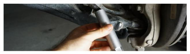
11) Thread tie rod end back onto tie rod the same number of times that it was removed in step 7
