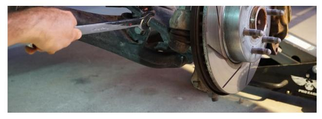
4) Using two wrenches, loosen tie rod joint nut but do not remove nut all the way
