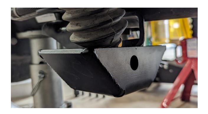
4) Insert bolt through shock skid, shock mount and shock
