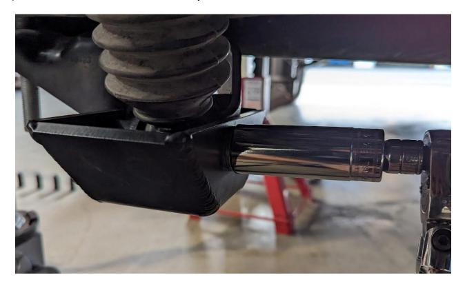
6) Using 22mm wrench mostly tighten nut onto back side of shock skid
