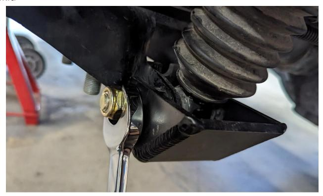
7) Follow with torque wrench and torque nut to 118 lb\*ft
