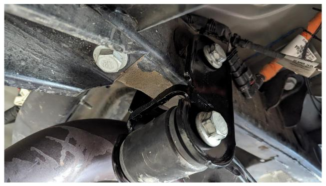
4) Using 21mm socket and wrench, remove the two bolts
