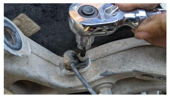
8) Use an 18mm deep socket to loosen the two brake caliper bolts, remove the caliper and hang it using strap (coat hanger/zip tie work also) being sure not to stretch the brake line
