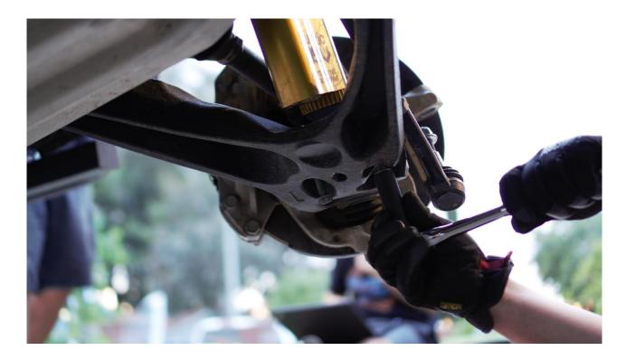
53) Reinstall the upper ball joint into the knuckle and tighten with 18mm wrench and 5mm allen, torque to 37 lb-ft then 90-110 degrees
