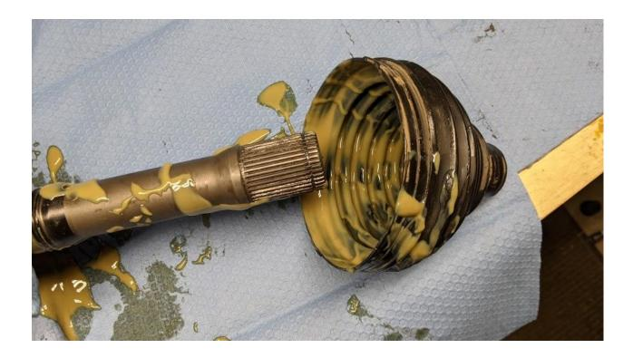
32) Thoroughly clean the inside and components on both ends of the cv and slide the new boot on
