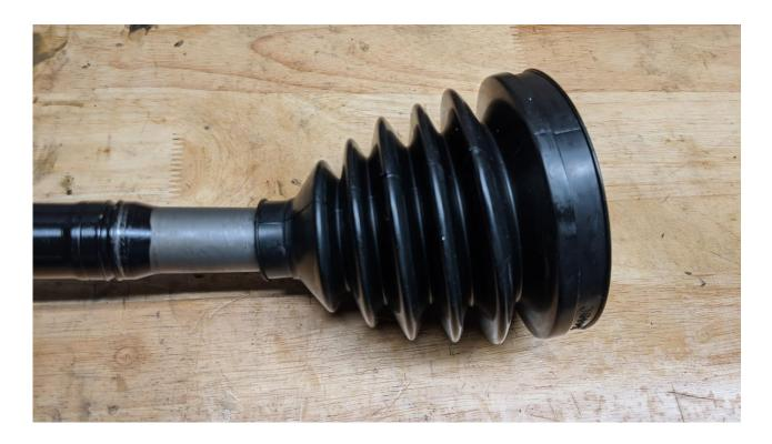
38) Make sure to line up the boot with the line on the axle shaft
