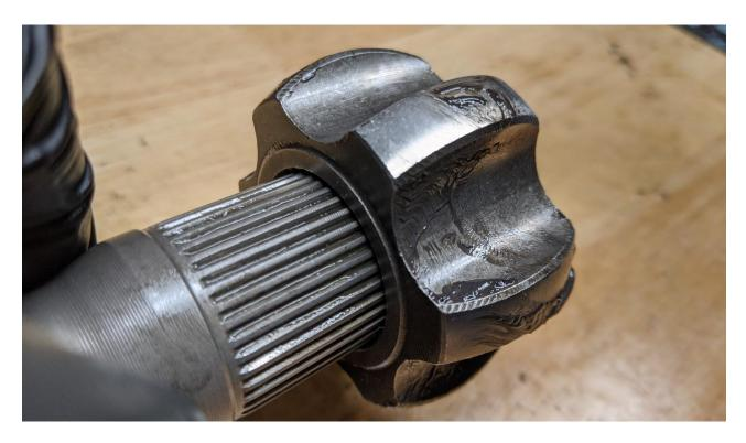
42) Slide the outer cage back over the inner
