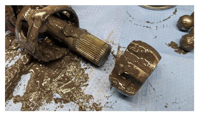
29) When removing note the orientation of the inner part, the side with the boss goes on first
