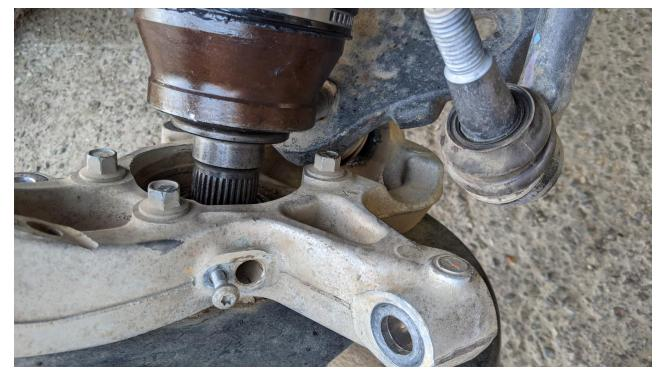
51) Tighten the 27mm nut on the lower balljoint and torque to 55 lb-ft and then 90-105 degrees
