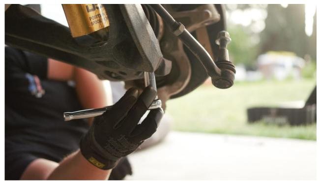
13) Loosen upper control arm ball joint using 18mm deep socket, you may need to use 18mm wrench and 5mm allen to avoid spinning the ball joint, DO NOT REMOVE all the way
