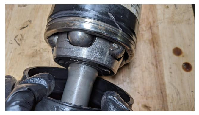
46) Reinstall the c-clip making sure it is fully seated in the groove, with the boot peeled back empty the rest of the second grease pack into the CV. You will need to pack the grease into the cage and balls making sure it is fully distributed. Failure to do so will cause premature wear.
