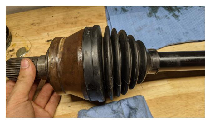
33) Be sure to line up the small end of the boot with the line on the axle shaft
