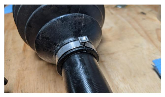
35) Pull the boot back and squeeze one of the packets into the cv and boot, thoroughly work the grease into the CV joint being sure it is well packed, failure to do so can cause premature wear
