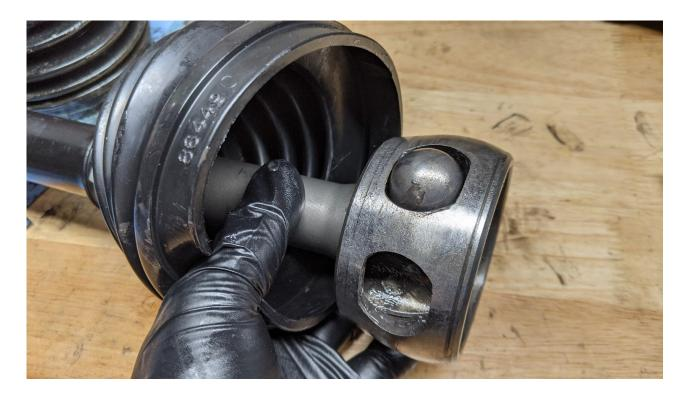
45) With the balls in place, slide the outer housing over the balls and cage
