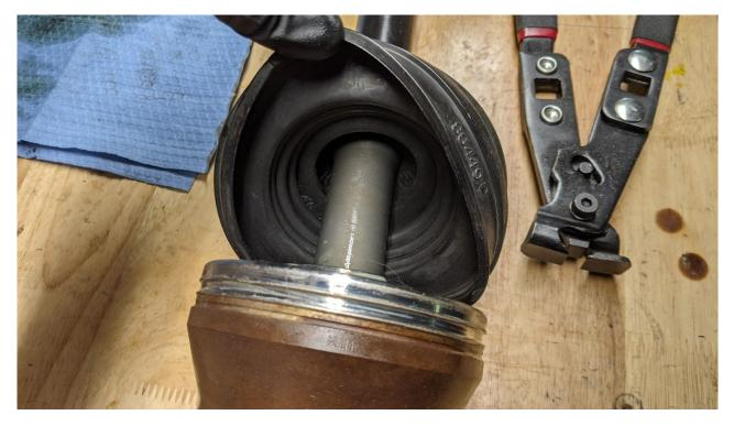
36) Place the large clamp on the axle and crimp using the correct tool, be sure to let out any excess air so the boot remains in a relaxed state
