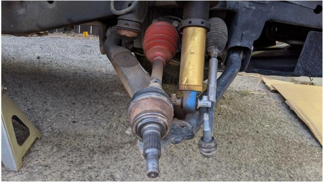
17) Next fully support the axle. Using a small prying device between the axle and the differential carefully pry the splines past the c-clip groove internally, remove the axle BE SURE TO NOT DRAG THE AXLE ACROSS THE SEAL
