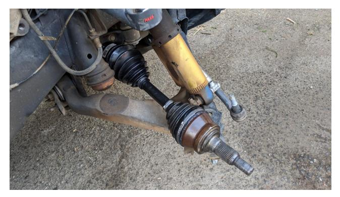
50) Reinstall the knuckle onto the lower arm while guiding the axle into the wheel bearing, it may be helpful to have people for this
