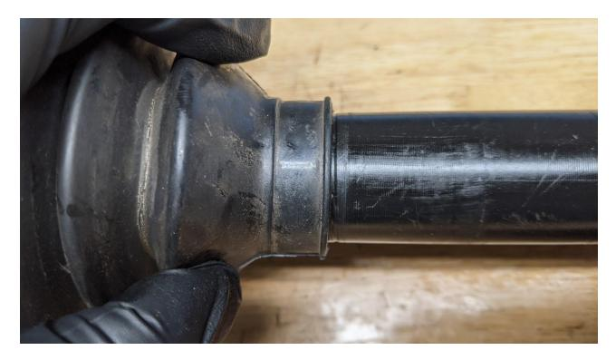
34) Place the small clamp on the axle and crimp using the correct tool
