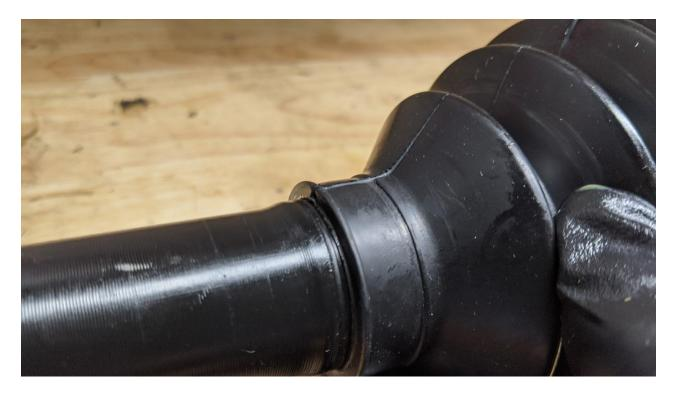
39) Install the small clamp and crimp using the correct tool
