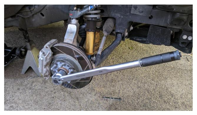
57) Reinstall and torque wheels58) Recheck all bolts after 100 miles of driving
