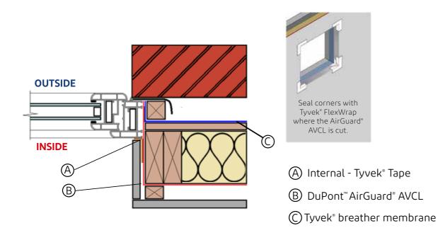
Fig. 4 - External wall insulation (EWI systems / ETICS)
