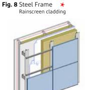
Fig. 9 Steel Frame 🔸 Rainscreen cladding - open joints
