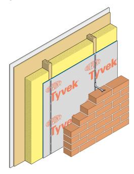
When timber and steel frame walls are internally sheathed, the sheathing board may provide the racking strength, contribute to fire resistance, comply with surface spread of flame (reaction to fire) classification and provide the internal decorative surface. Such boards may include cementbonded particleboard, fibre reinforced gypsum board, mineral fibre boards, and fire retardant treated plywood, OSB and chipboard.
