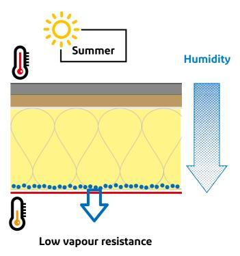
Excessive moisture trapped in the construction can evaporate to the inside
