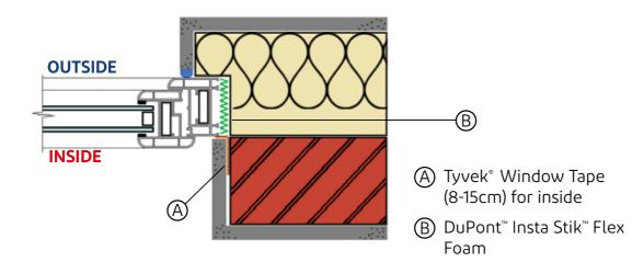
\* NOTE: Some external sealing provisions may not be necessary if the external insulation is being fitted immediately after the window unit.
