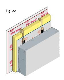
An internal air & vapour control layer (AVCL), such as DuPont<sup>™</sup> AirGuard<sup>®</sup> Reflective should be installed with meticulous attention paid to all laps, edge details and penetrations. Sealing the AVCL in this system is key to the prevention of condensation on the inside face of the existing wall.
