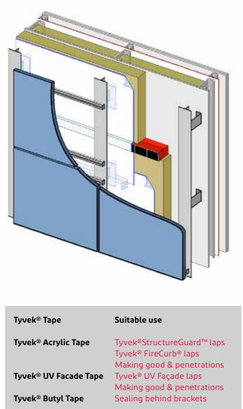
The Tyvek<sup>®</sup> membrane should be dressed over fire barriers that are fitted around windows. This will maintain the integrity of the window opening for air sealing and weather tightness. The normal recommendations for lapping and tape sealing apply.
