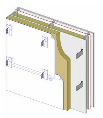
• Above: Laps in Tyvek<sup>®</sup> StructureGuard and Tyvek<sup>®</sup> FireCurb<sup>®</sup> breather membranes are sealed with Tyvek<sup>®</sup> Acrylic Tape.
