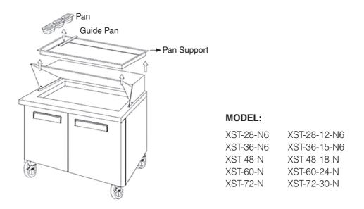
1) Remove the Guide Pans and Pans. Then pull out the Pan Supporter. Clean the pan supporter and reinstall in place.
