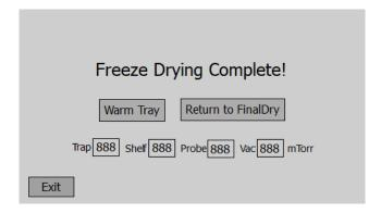
Step 3: If the food requires further drying, return the trays to the freeze dryer and close all valves. Press the 'Return to FinalDry' button to access the following screen. Press the 'INC' button to add additional drying hours (e.g., 4 hours). Once the 'Final Drying' button becomes available, press it to restart the drying process.
