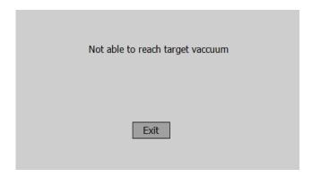
If the vacuum pressure reading does not reach the benchmark values at different points, a warning will appear when the vacuum pump is started. To return to the freezing mode screen, press the 'Exit' button.
