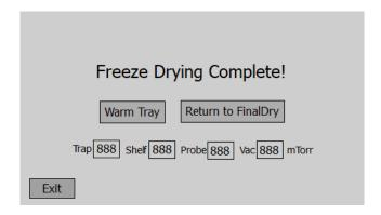
Open the vacuum valve and wait for the pressure to be normalized in the chamber. Open the door to check if the food on each tray is completely dry. If not completely dry and the food is still frozen, put the trays back, close the door and press 'Return to FinalDry.' The screen will jump to <a href="https://example.com/Auto-finaldry-pause">Auto-finaldry-pause</a> screen. Follow the instructions on <a href="https://example.com/Auto-finaldry-pause">Auto-finaldry-pause</a> screen to resume drying.
