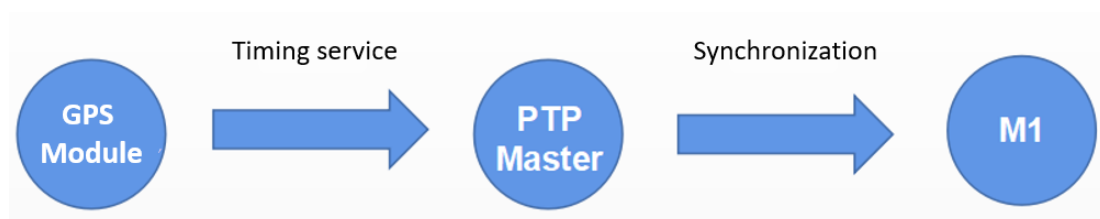
Figure 4: Topology of GPS Timing service synchronization
