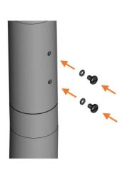
25. Using a spirit level and phillips head screwdriver, adjust the angle of the heater head to be level by adjusting the 4 x Dome Head screws (M4 - Length: 6mm) on the heater head.
