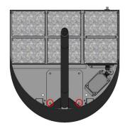
11. Fasten the **rear** two slots of the Lower Arm section to the Base using 2 X M8 Washers, and 2X M8 - Length: 35mm bolts.
