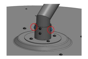
18. Fasten the 4 X Dome Head Screws (M4 - Length: 6mm) to the head to lock the angle of the Heater Head relative to the Top Arm section.
