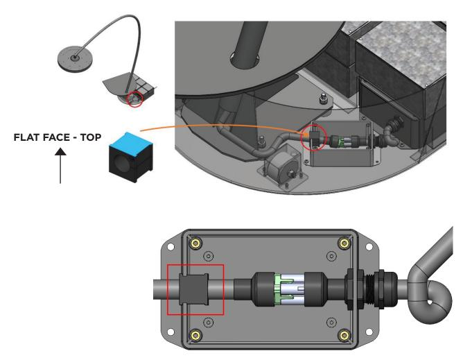
29. Fasten the Small Connector Box lid using the 4 X Oval Head Screws (#4-40 - Length: 3/8")
