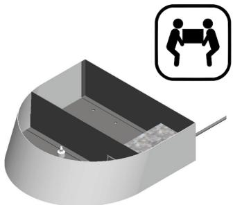
6. NOTE: If installing in areas subject to high winds, gusts or hurricanes, heater base must be bolted down to ground using appropriately sized and type bolts (not included) suited for the ground surface through the 5 X Holes in the Heater Base.
