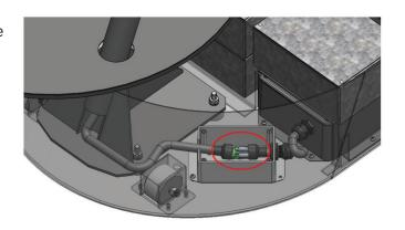
28. Attach the rubber cable grommet around the cable, and place it in the square slot in the connector box, ensuring the flat face is facing upwards.
