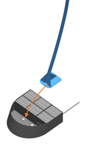
Fasten the **front** two slots of the Lower Arm section to the dampeners using 2 X M8 Washers, and 2X M8 Nuts.
