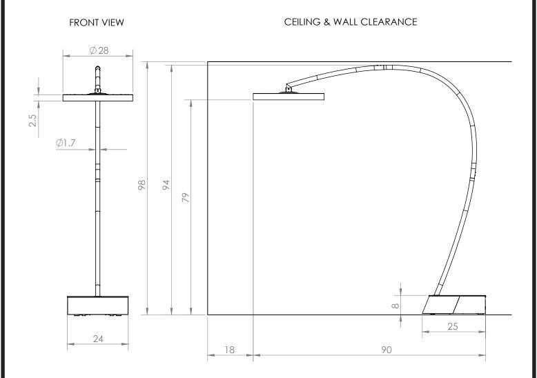
The stated clearance to combustible materials represents surface temperature of 117°F above room temperature. Building & other structural material with a low heat tolerance (such as plastic, vinyl siding, canvas, tri-ply etc.) may subject to degradation at lower temperature. It is the installer's responsibility to assure that adjacent materials are protected.
