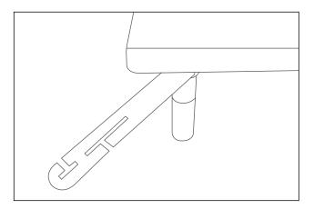
2 Slide side (a) of the connecting strap onto leg bolt. Swing the strap and connect side (b) to the leg bolt. Secure the strap by shifting to the left.
