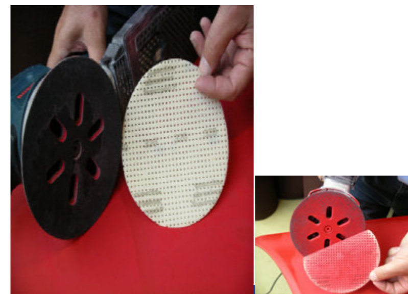
Example of use before/after: Dust extraction Superpad P Gold, grain 320 with random orbital sander Ø150 mm
