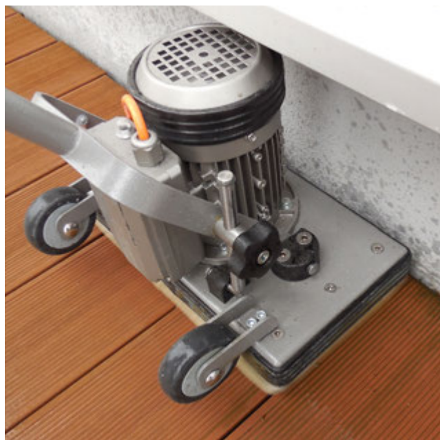
Cleaning of WPC (wood-plastic composites) terrace boards with the Jöst Floor Sander Junior and microfiber pad blue/melange
