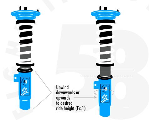
Divorced spring setup will rely on spring perch collars for height adjustment.
