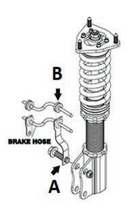
Included are (4) moldable brake line/ABS brackets (A) with rubber grommets (B) for applicable applications. These brackets may be modified to meet the required configuration.
