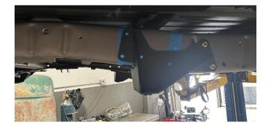
Bolt the bracket to the two rearmost holes for the front leaf spring hanger. Push the tab of the bracket up against the bottom of the frame as you tighten the two M10 bolts and nuts.
