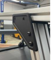
Measure the amount of crossbar sticking out on each side of the upright assemblies. Try to move the crossbar to get these measurements as close as possible to center the crossbar. Once once centered, install the drop in T-nuts into the crossbar channels. Slide nuts into position untill they are aligned with the holes on the corner plates. Apply blue loctite to the supplied 5/16"-18 x 5/8" bolts and thread into the t-nuts. Snug bolts.
