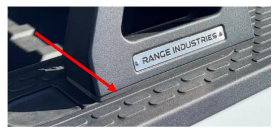
Use two of the supplied  $5/16''-18 \times 1''$  stainless steel bolts to mount upright to the anchor point. We recommend the use of blue Loctite on all hardware for this install. Snug the bolts down until the upright is standing up fully. Push the base of the upright forward toward the opposite side of the bed while tightening. This makes the upright register off the vertical surface of the anchor point and keeps the upright square to the bed. Repeat this for the other upright.
