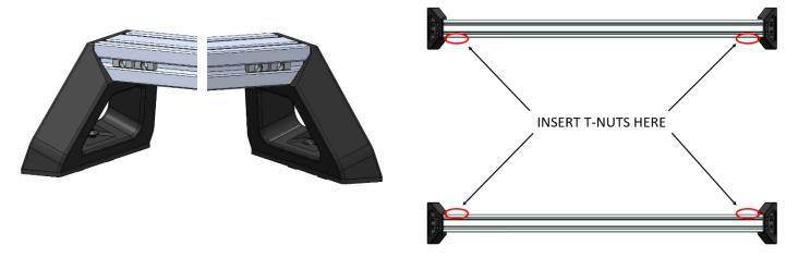
Next we are going to assembly the molle panel sub assemblies. Begin by installing 4x T-Nuts in each of the molle panel support rails.
