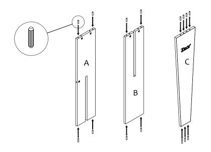
STEP 2 Screw the feet Type F into appropriate holes
