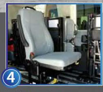
Our Step N Lock latching mechanism will only work if the seat is installed 100% into the track, eliminating operator error.
