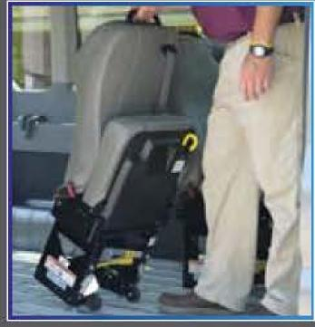
AbiliTrax provides drivers with a much more user friendly environment when they are changing seating configurations. By the driver simply using their foot, AbiliTrax allows for "hands free" latching and unlatching of the "Step N Lock" seat base.
