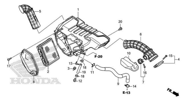
The goal of this guide is to install the high flow velocity tube into the CRF 300L Airbox. This part replaces part number 6 in the diagram above. To accomplish this, please follow the below process:
