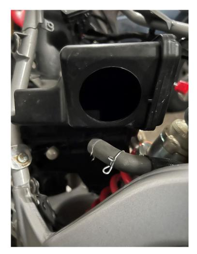
36. Open the airbox tube hole to <u>62mm [2.44"]</u> in diameter
