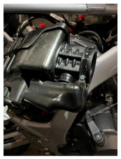
38. Install the new high flow velocity tube into the airbox
