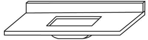
Countertop and backsplash
