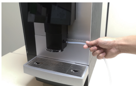
1.Connect milk pipe to machine
