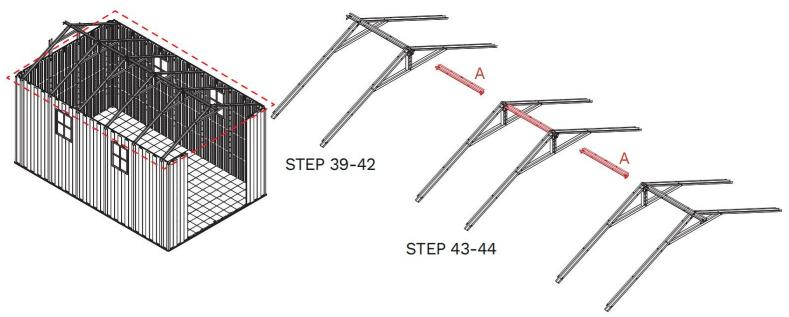
Beam installation can be divided into three groups: the installation steps for the front and rear components can be found in STEP 39-42, while the installation steps for the middle components are detailed in STEP 43-44. Install the front and rear components first, then install the middle components. When installing the middle components, please use your hands to support Area A.
