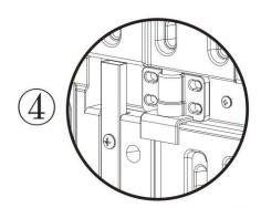
After inserting the DDZ, push the DR and DL to the fitting position.
