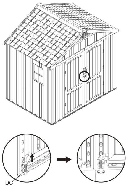
Remember to unplug the DC when closing the door and put it down when the door is closed.
