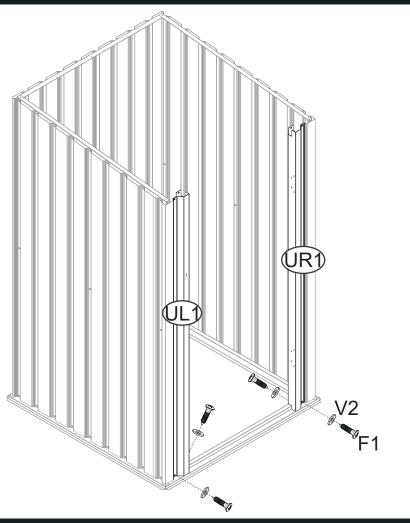
UL1and UR 1There are holes on the inside and outside. All need to be fixed with screws.
