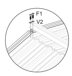
**Note:** Do not install F1 and V2 in the holes near the outer side of P1,P2.
