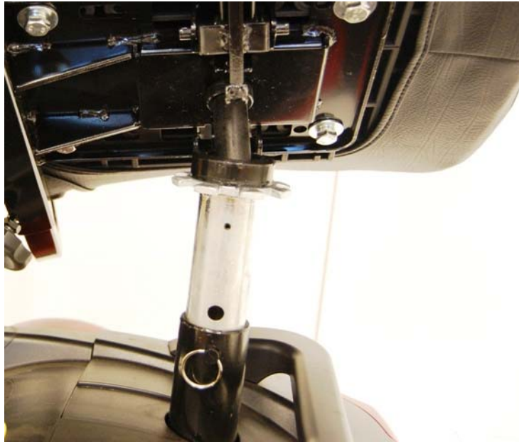
Figure 23. Installing the Seat
