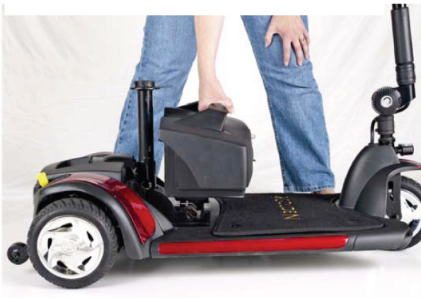
Figure 21. Battery Pack Installation
