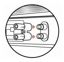
Loosen reservoir cap and then press drain key into the control unit's connector to drain the reservoir. Don't turn the control unit upside down to empty the unit. It will damage your appliance and void the warranty.
