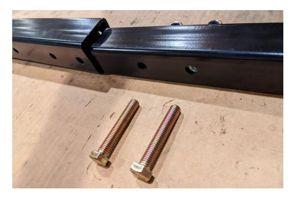
Insert upper vertical into lower vertical. Thread bolt 1 into the **spring nut side** and tight the bolt to the spring nut to remove all play first. Then add bolt 2 and both nuts and tighten fully. Do not use bolt 2 for fully tilting plates.
