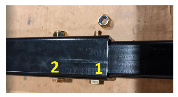
Now your Chuck BASE post assembly is complete. Tighten bolts as needed to increase the friction of the tilt assembly.
