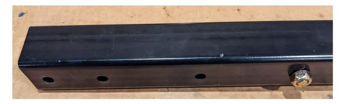
For full tilting ability with a Chuck Bucket move the above bolt one hole to the left(3rd hole). This will allow for clearance of the bucket to the lower plate.
