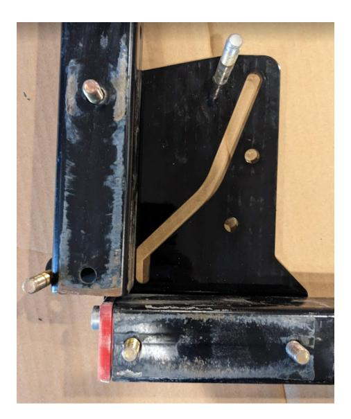
Place the other side plate on top of the assembly and add washers and nuts finger tight.
