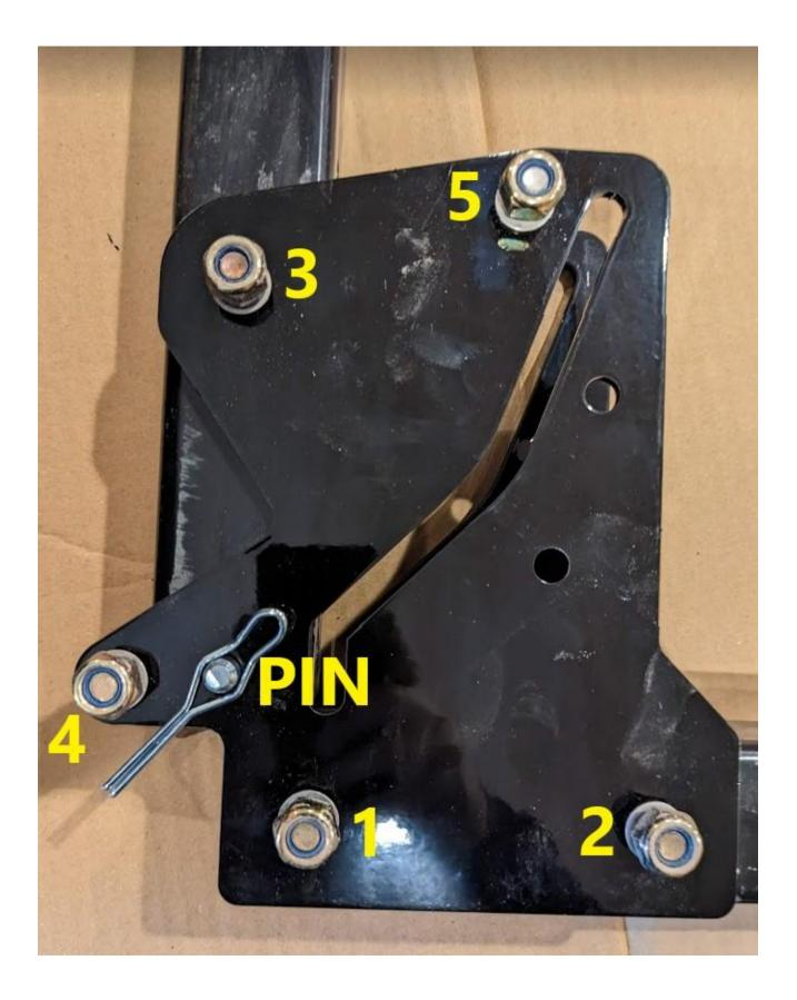
Insert locking pin as shown and tighten bolts 1 and 2 very tight (40 Nm recommended). Tighten Bolt 3 until snug. Note that this can be tightened further to increase tilt mechanism friction. Finally tighten over travel bolts 4 and 5 until they are no longer loose. Do not over tighten bolts 4 and 5 or the unit may have difficulty tilting.
