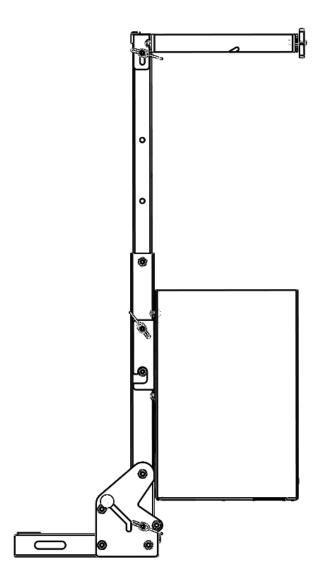
Insert and secure the locking pin into the lower tilt mechanism. **Note the lower tilt mechanism is not secure without the lower locking pin in place. Accidents may occur.** Spontaneous rearward tilting can and has occurred over large bumps. Chuck Rack LLC is not liable for accidents due to inadvertent tilting when the locking pin is not present. Be Advised.
