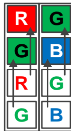
Figure 8-48 Vertical color Binning by 2
