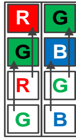
Figure 8-39 Vertical color Binning by 2
