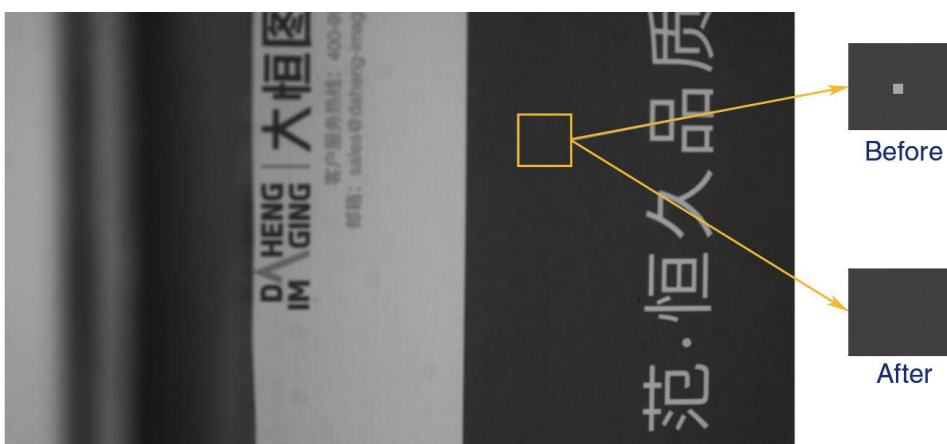
Figure 8-60 Defect pixel correction effect in actual scenario
