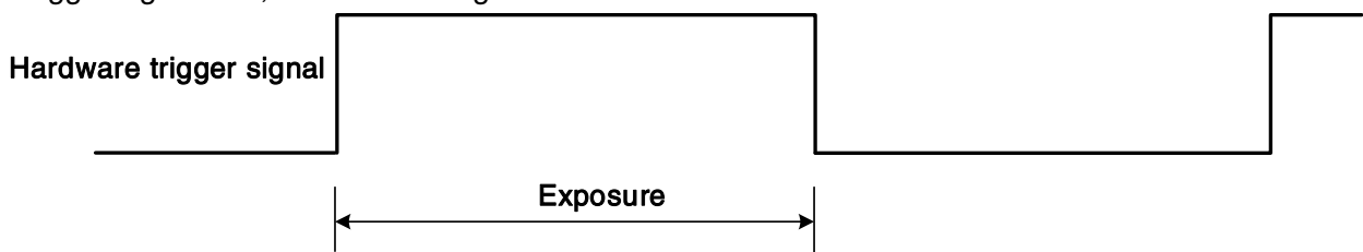
Figure 8-25 The sequence diagram in rising edge trigger of TriggerWidth exposure mode
