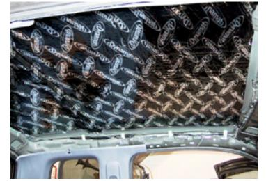
**Dynamat Xtreme** is very simple to cut and install. The butyl rubber and heavy aluminum will stretch and contour better than any other product on the market without tearing. It will conform easily to all interior surfaces, and the sticky butyl rubber will adhere to a surface and stay in place without any special surface prep, and without leaving any odor or dripping material. Install it in your vehicle, and experience the Dynamat Difference.
