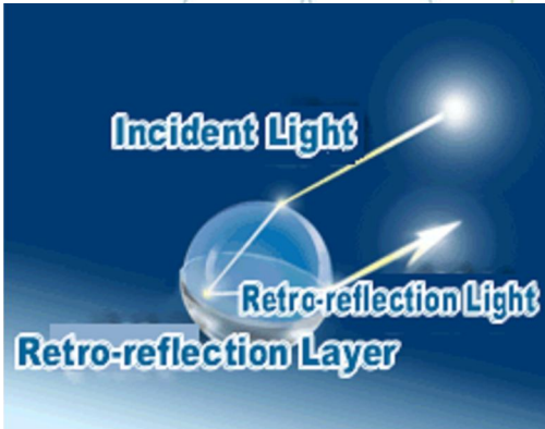
Figure 5: Inverse Retro-reflection Principle of Micro-prism Type Retro-reflection Sheeting
