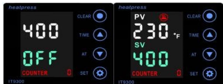
Heat press enters into power off , mode if machine is kept quietly for set time and without any operation User can wake up heat press and start heating by touching any key
