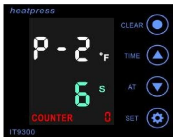
P-2:Time Setting Mode. Touch SET & ↑↓ keys to set desired time
