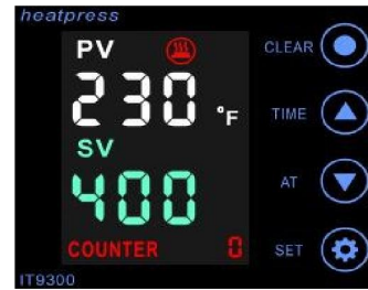
P-1:Temp. Setting Mode. Touch SET & ↑↓ keys to set desired Temp
