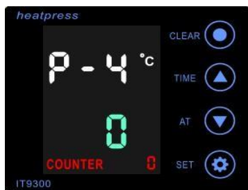
P-4: Auto Power-off Mode Touch SET & keys to set auto-off time with 0~120 min range
