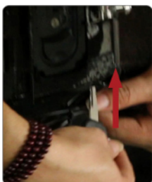
3.Insert the key to battery lock
