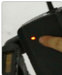
4.Red Light shows the battery is charging, green light is full
