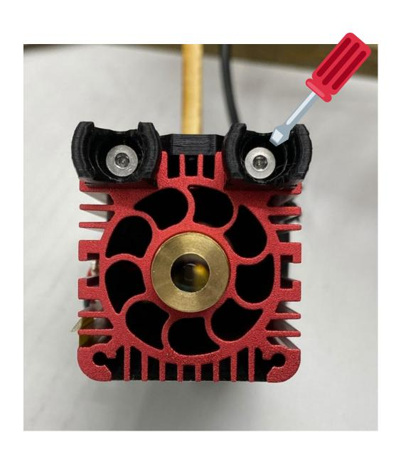
Note - If you are using our King Gubby Z Axis Adjuster with this Air Assist, make sure that the Z Axis's Module plate is positioned high enough to allow for the brackets to sit flush.
