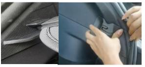
2.Attach the two cargo cover hangers to the rear seat headrest stays as shown.
