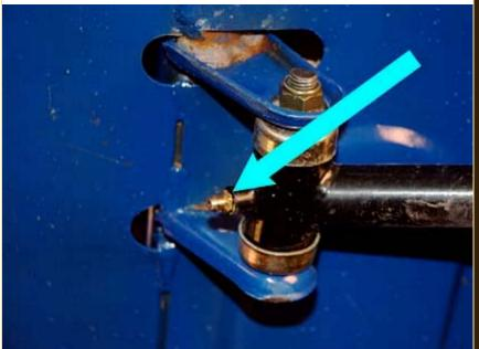
Note the grease nipples on each lower control arm pivot and always remember to keep them properly greased.
