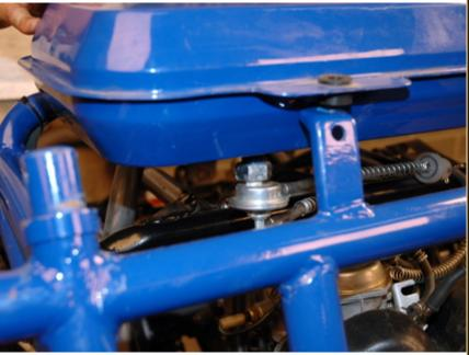
Now rest the fuel tank on it's mounting brackets.
