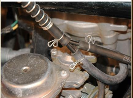
Next, connect the fuel petcock's vacuum line to the engines vacuum Y-connector.
