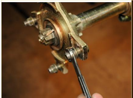
Now remove the lugnuts from the rear hubs.
