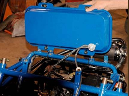
This is the correct way to install the 2007-model-year fuel tank.
