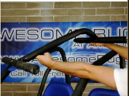
Now for the rollcage H-bar. This is how it should be positioned.
