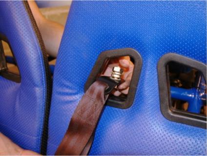
Now feed the harness top mounting point through the innermost of the 2 holes in the seat back.
