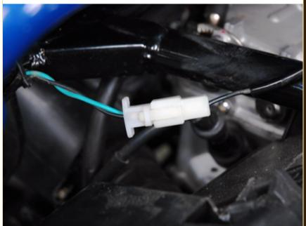
Next, plug the radiator fan wire into its matching connector on the chassis wiring harness.
