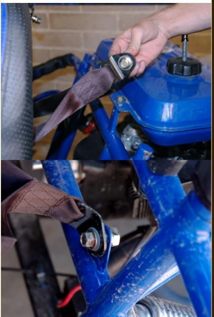
Finally, take each shoulder harness anchor and, using the same hardware order as you used for all the other mounts, attach them to their mounting points on the chassis.
