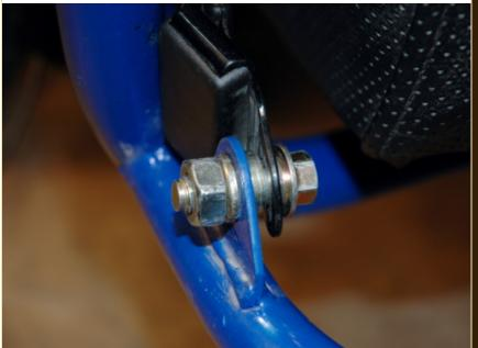
This is how the seatbelt ends should look after tightening.
