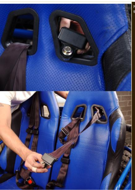
Now feed the outer harness and seatbelt half through the outer hole in the seat back.
