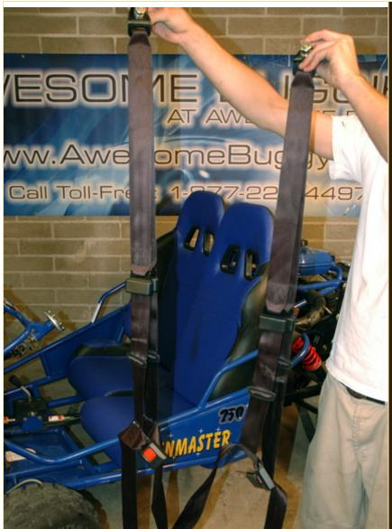
The seatbelts for each occupant are joined in the center and share a common mounting point on the chassis, so follow these steps carefully.
