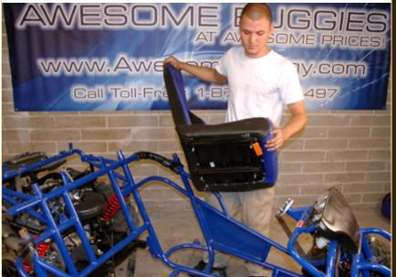
First, find the driver's seat. This is the one with the side bolsters towards the driver's side of the buggy.
