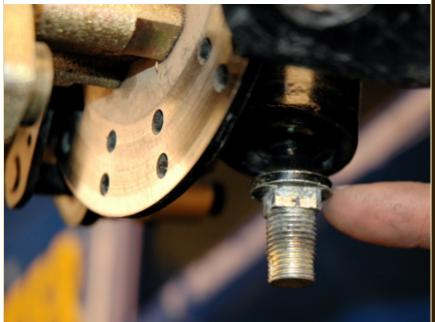
This is the mounting stud for the lower balljoint on the steering spindle. Note the square area above the threads.
