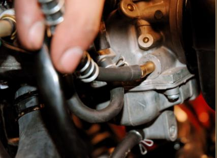
Now connect the fuel line (the one with the filter in it) to its nipple on the carburetor. Clamp the hose to the nipple with the butterfly clamp provided.
