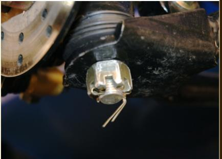
Now insert one of the provided cotter keys into the hole in the stud and bend the ends back so it will not fall out.
