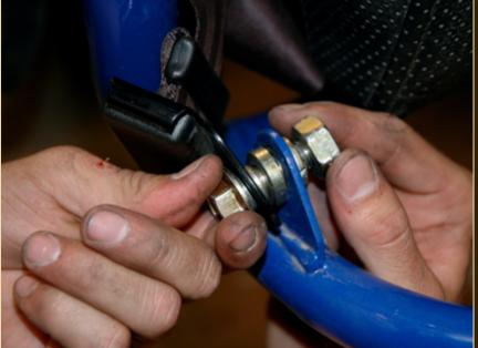
This is the order for the hardware used to mount all the seatbelt and harness ends.
