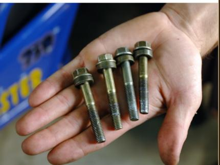
Insert these bolts through the longitudinal bars and thread them into the ends of the H-bar.
