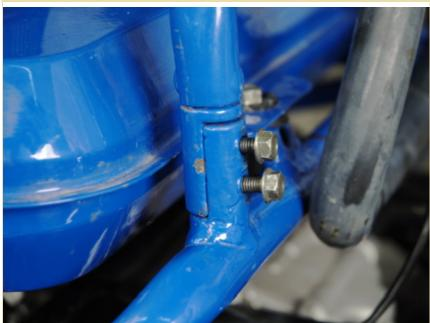
Take your radiator and align it with its mounts located just in front of the fuel tank.
