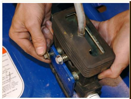
Next, thread 2 of the bolts through the chassis mounts into each of the lever housings and tighten them.
