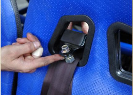
Feed the entire driver's side outer harness and seatbelt through the hole, as well.
