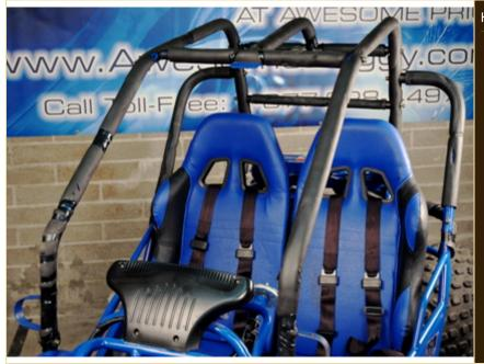
Here is the rollcage completely installed.
