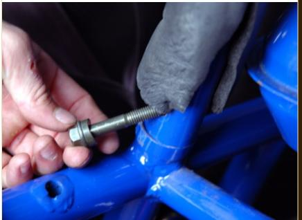
Insert the rollcage bolts and start the nuts on them, but do NOT tighten them at this time.
