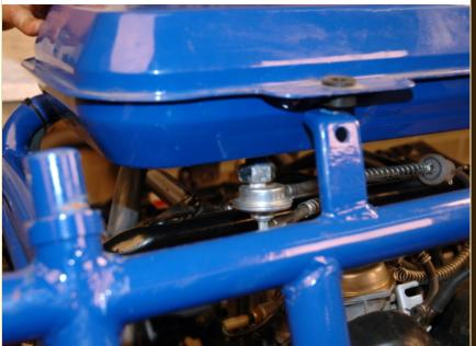
The front passenger-side tank bracket comes from the factory slightly out of position and this prevents the mounting bolt from threading properly into its threads when the others have all been installed properly.
