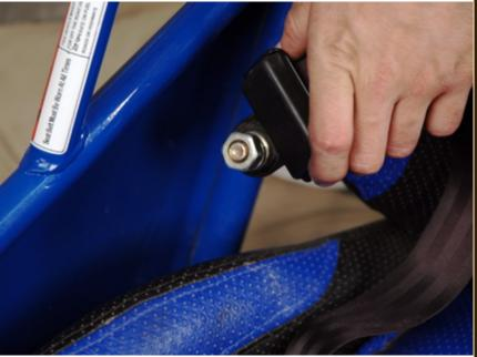
Now take a seatbelt or harness end and attach it to the chassis. We started here with the outer passenger seatbelt mount.
