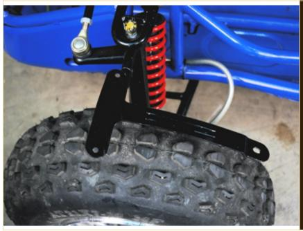
First mount the front fender bracket to the front steering spindle.
