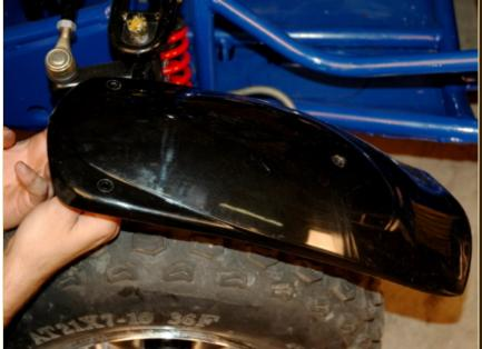
Then bolt the front fender to the bracket.
