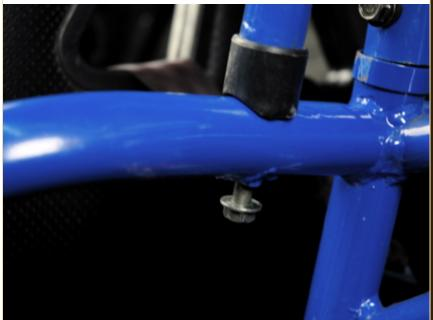
Finally, thread the front mounting bolts into the front ends of the rack and tighten them.
