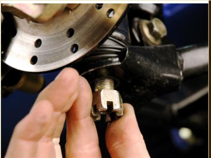
Once the stud is properly seated into the lower control arm, thread on one of the castellated nuts onto the stud and tighten it.
