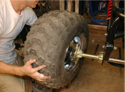
Place the rear tires/wheels on the hubs, then thread the lugnuts onto the lugs and cross-tighten them.
