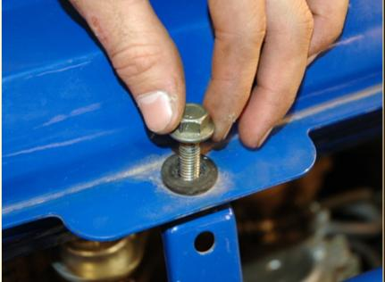
Now thread 3 of the bolts into their brackets. Do NOT insert the front passenger-side bolt yet!
