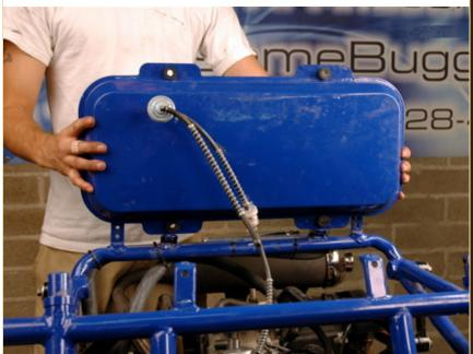
This is the RIGHT way to install the pre-2007-model fuel tank.
