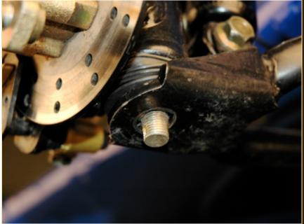
Insert the lower balljoint stud into the square hole on the lower control arm. Ensure that the square portion of the stud is seated all the way into the square hole on the control arm. Turn the front spindle to align these as necessary.
