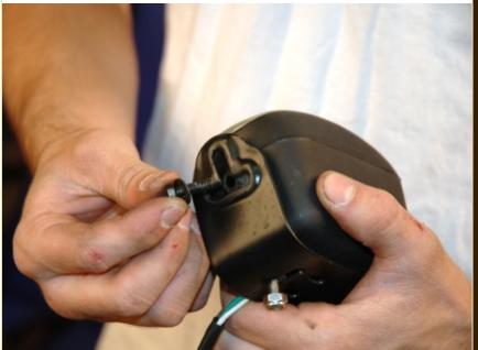
Remove the headlight pivot screws from each headlight.
