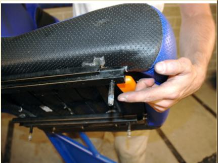
Move the seat rails until both are either fully to the rear or fully to the front. Then take the seat and place it in the buggy so that the seat rail studs go into their respective mounting holes in the chassis.
