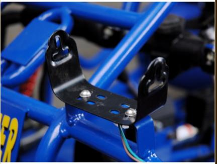
Place each headlight into a bracket, then thread the pivot screws into the headlight. Do NOT tighten them all the way, but tighten them enough that when you aim the headlight, it will hold its position in the bracket.
