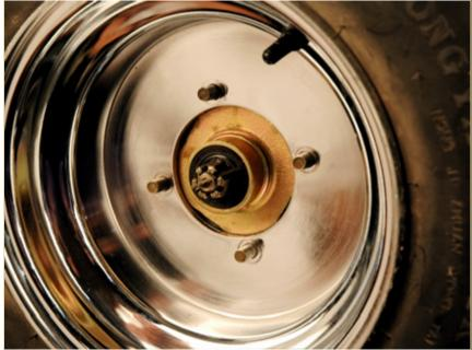
Once the front suspension is properly put together, remove the lugnuts from the front hubs, mount the front wheels/tires, reattach the lugnuts and cross-tighten them.
