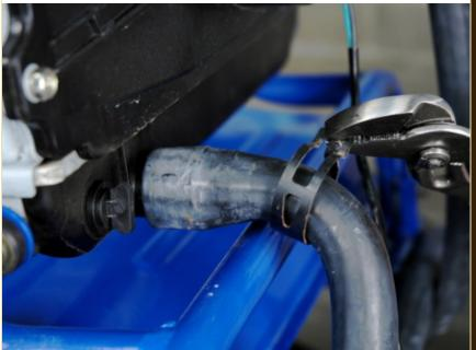
Now push the radiator hoses onto their respective nipples on the radiator. Use a pair of pliers to place the radiator hose clamps over the nipples.
