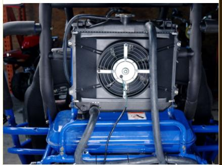
This is what a correctly installed radiator should look like.
