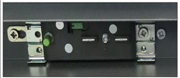
When the correct height has been confirmed by the green catch clicking, the soft close function closes the door correctly with no gaps the activator can be secured to the top track using 2 x 20mm screws.
